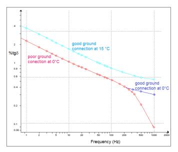
Fig. 6. Measured curves of the transformer at different conditions and poor/good ground by FDS method and apparatus IDAX-350.
