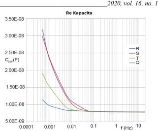
Fig. 8. Comparison of the measured autotransformers R, S, T, Q according to the real capacities for connection high-voltage winding – tank  $C_{\rm HT.}$
