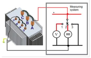
Fig. 1. Principal scheme of the RVM method.
