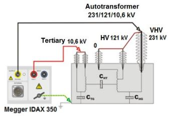
Fig. 7. Connection of the instrument MEGGER IDAX-350 to the measured autotransformer 231/121/10.6 kV.
