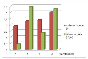
Fig. 10. Comparison of measured autotransformers R, S, T, Q according to the moisture in the paper (%) and oil conductivity (pS/m).
