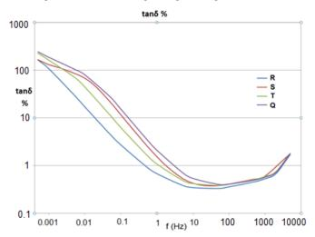
Fig. 9. Comparison of the measured autotransformers R, S, T, Q according to the percentage dissipation factor (tg8 %) depending on frequency.
