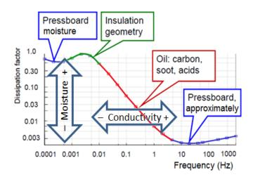
Fig. 3. Analysis of insulating transformer properties by the curve of FDS method.
