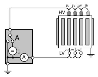
Fig. 2. Principles of an easy PDC system.
