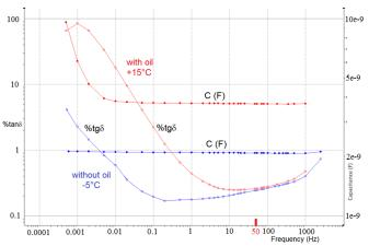
Fig. 5. Measured curves of the transformer at different conditions by FDS method and apparatus IDAX-350.
