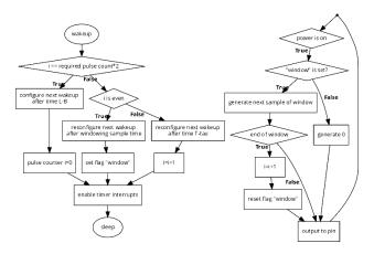
Fig. 3. Flowchart of windowing function in MCU.
