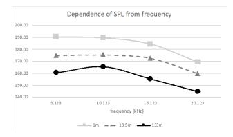
Fig. 7. Dependence of the average sound pressure level on the frequency at various distances between the speaker and the hydrophone.
