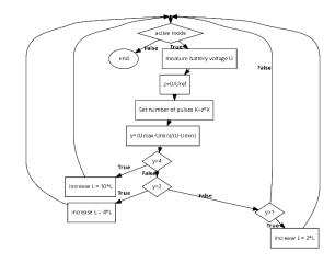
Fig. 4. Algorithm for adjusting signal parameters according to the battery level.
