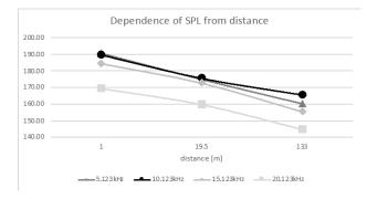
Fig. 8. Dependence of the average sound pressure level on the distance between the speaker and the hydrophone.
