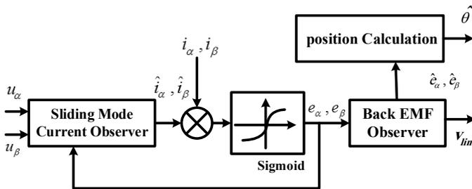
Fig. 3. Block diagram of the proposed sliding mode observer (PSMO).
