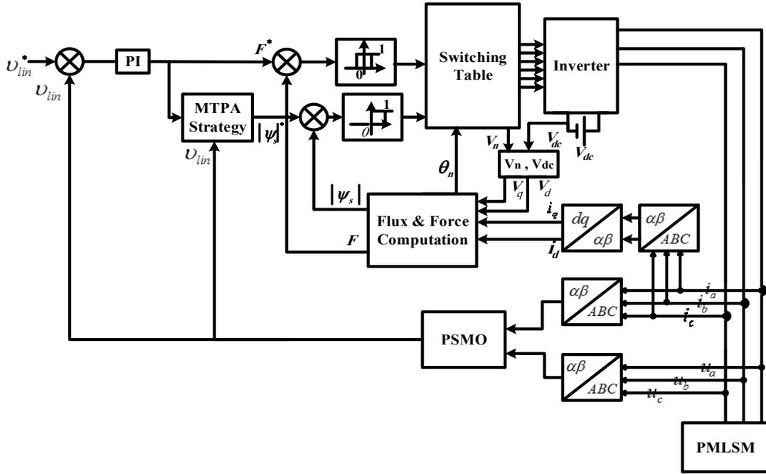
Fig. 2. Block diagram of the PMLSM sensorless control.
