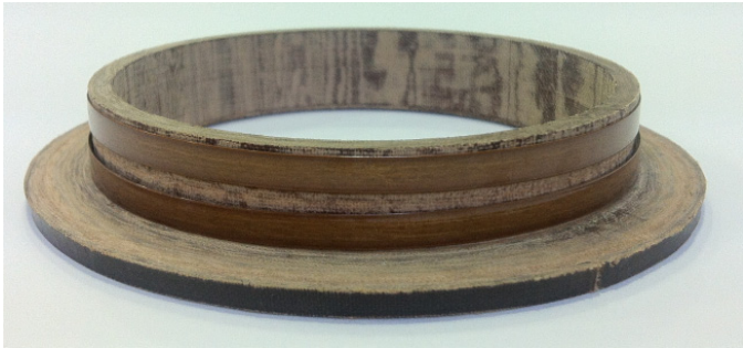
Fig. 3. View of the secondary, built by two first generation superconducting tapes wrapped around a Celeron holder.
