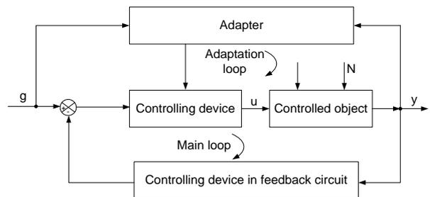
Fig. 4. Structural scheme of adaptive system.
