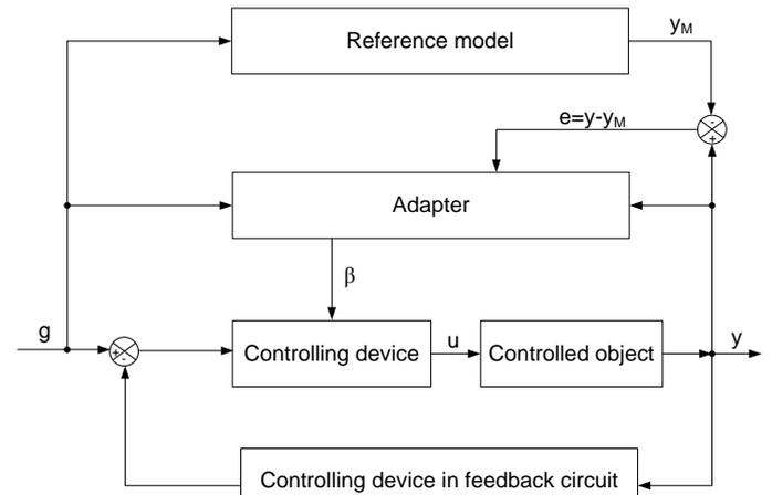
Fig. 5. Structural scheme of adaptive system with reference model.
