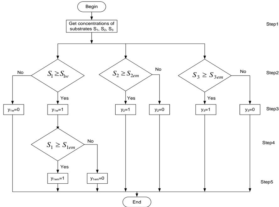
Fig. 9. Algorithm of biosensor control system.
