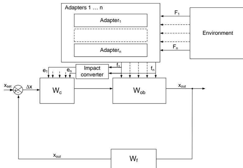
Fig. 6 Structural scheme of adaptronic system.
