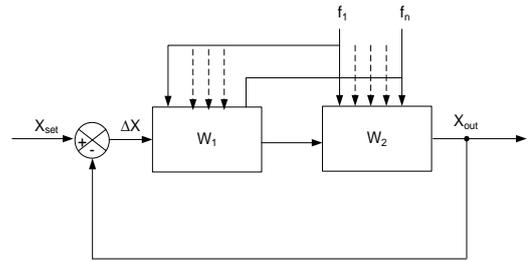
Fig. 3. Structural scheme of self-tuning ACS [11].
