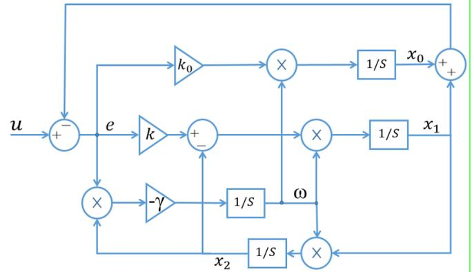
Fig. 2. Schematic diagram of the notch filter.
