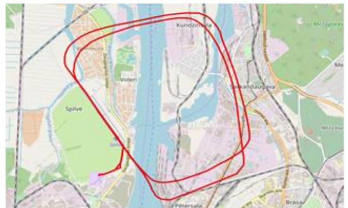
Fig. 2. Visualized GPS coordinates of the horizontal flight path.
