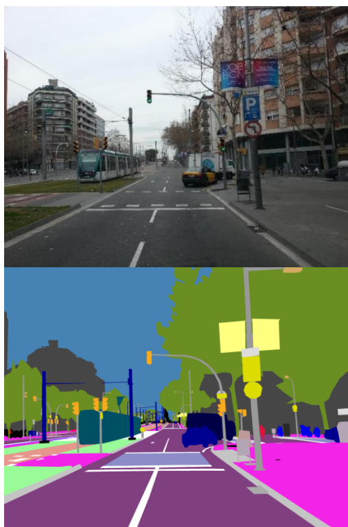
Fig. 1. An image which is to be semantically segmented and the result of segmentation [7]. There are a few tens of classes of labeled pixels, and each class is shown with its own color. Some colors are chosen in accordance with real tints of the corresponding objects or scenes (for instance, the trees in this example are labeled green, although there is no verdure due to a specific season). This is an example of a very accurate complex segmentation.
