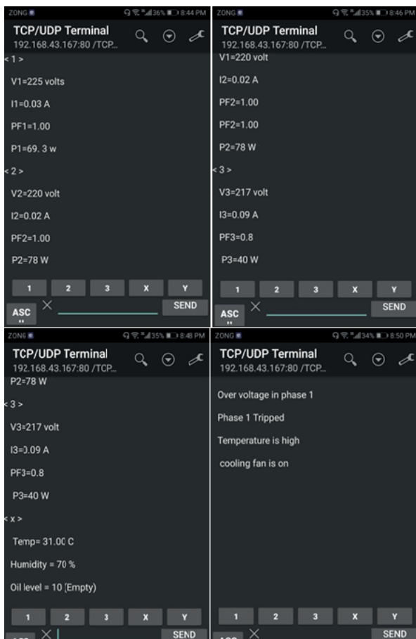
Fig. 15. Results of the system in the android application (TCP/UDP Terminal).
