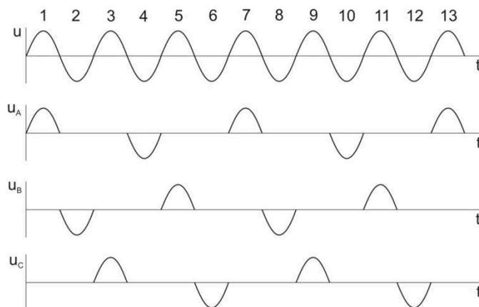
Fig. 1. The distribution of stator windings voltages
