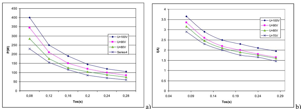
Fig.3. Consumed power  $P$  and current  $I$  dependent on oscillation period  $T_{os}$ : a)  $P = f(T_{os})$ ; b)  $I = f(T_{os})$
