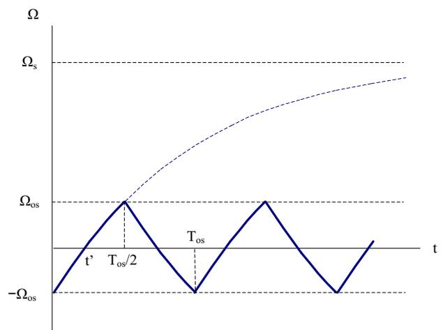
Fig. 2. The changes of rotation frequency in oscillating regime
