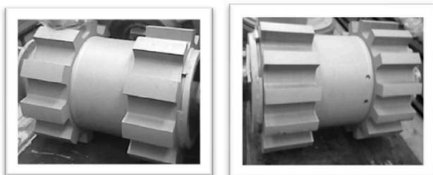
Fig.5. Rotors of generators: a - serial  $Z_2=10$ ; b - experimental  $Z_2=14$ .
