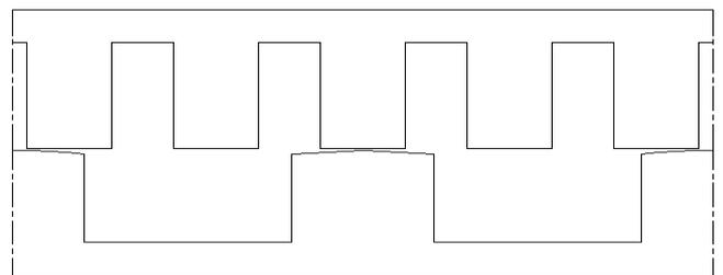
Fig. 2. Tooth zone of serial inductor generator with  $Z_1/Z_2 = 24/10$  and  $\gamma = 1.45$ .
