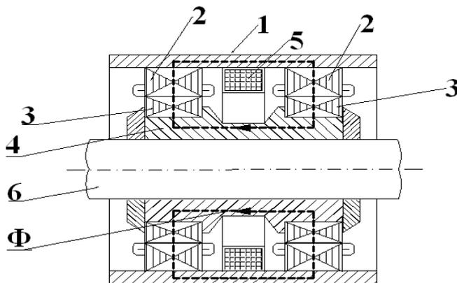
Fig. 1. Two-core axial inductor machine: 1 – body, 2 – armature cores with windings, 3 – rotor cores, 4 – rotor sleeve, 5 – excitation winding, 6 – shaft, ( $\Phi$  is a magnetic flux).
