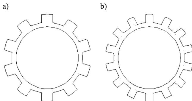
Fig.4. Sheets of the rotor: a – serial generator  $Z_2=10$ ; b-experimental generator  $Z_2=14$ .
