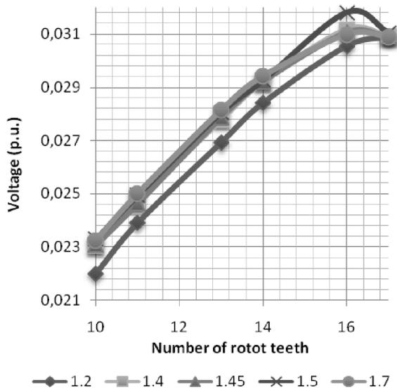
Fig.3. Voltage vs. the number of rotor teeth for relative slot width  $\gamma=1.2; 1.4; 1.45; 1.5; 1.7$ .
