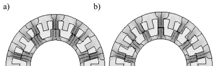
Fig. 8. Cross-section of magnetic field a - generator with tooth ratio 24/10; b - generator with tooth ratio 24/14.
