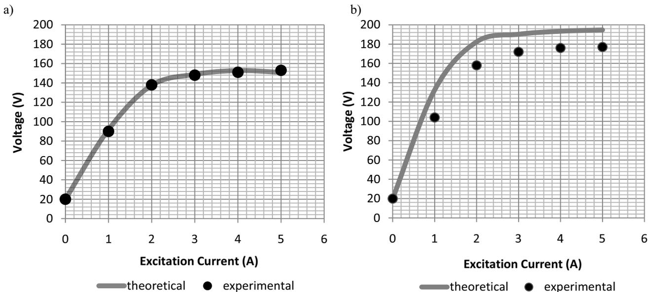
Fig. 7. No-load characteristics: a - serial generator  $Z_2=10$ ; b - experimental generator  $Z_2=14$ .
