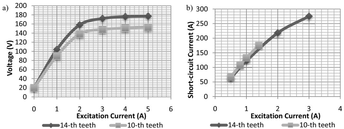
Fig. 6. Experimental characteristics: a - no-load characteristics of  $n = 950$  RPM; b - short-circuit characteristics.
