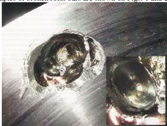
Fig. 1. Defective casting of a rotor bar of an induction machine [3].
